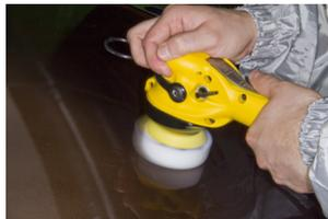
Polish the sanded surface for 5–10 seconds with suitable Mirka 77 mm foam pad using Mirka® ROP2-312NV machine.
