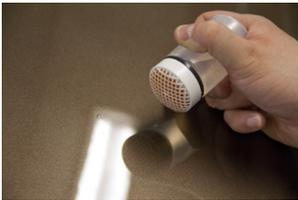
Use Mirka Damper to apply the right amount of sanding liquid.
